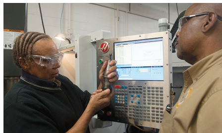
MCC student Vincent Owens, left, assembles a tool holder for a drill used in a CNC milling machine while his instructor, Anthony McCollough, watches.
