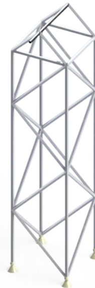
FIGURE 3.1: 3D MODEL OF DESIGNED TRUSS TOWER
